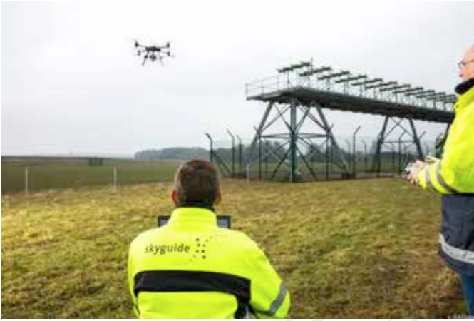
Drones can be used for regular maintenance of landing and navigational aids
