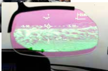
The Gulfstream G800 cockpit, and its Head-up Display (HUD) that shows the terrain ahead.
