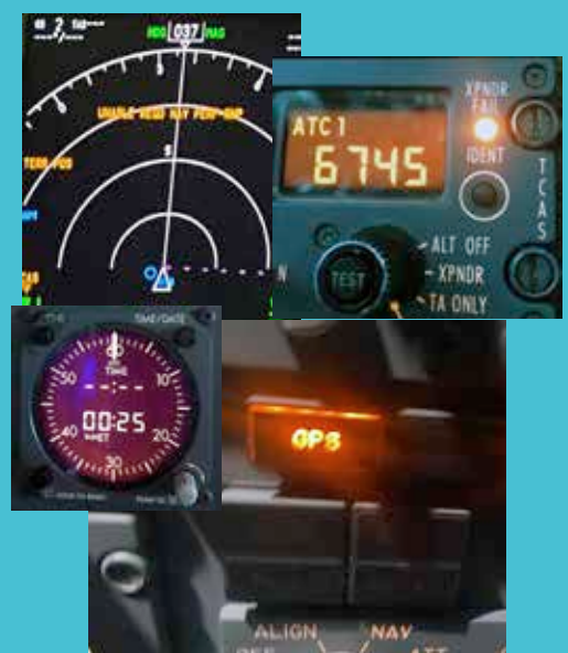
The different instrument indications in the B737-800 when the GPS signal is lost/jammed.
